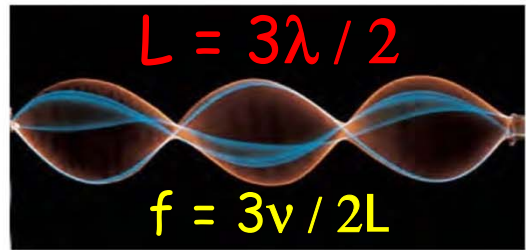
(c) String is one and a half wavelengths long.
